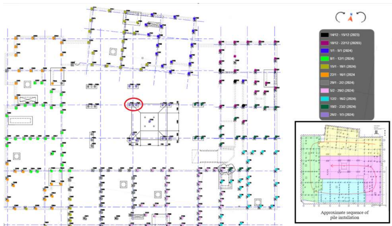
Figure 3.4: Pile installation reported per week at Brf. Sydney, the figure was generated with knowledge from profile about installation dates and the technical drawing, K-15-1-0080 .
